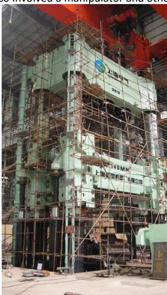
Figure 6. Scaffolding around the assembled CKV 120/140 SUNAN press prior to final assembly operations
