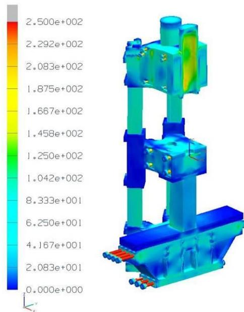
Figure 3. Stress distribution in the press frame after optimization (the model only comprised 1/2 of the frame)
