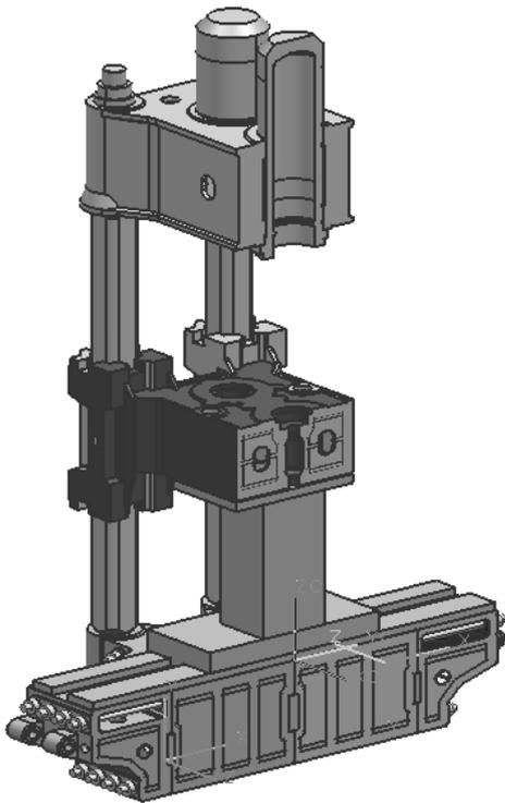
Figure 2. Model of one half of the CKV 120/140 SUNAN press
