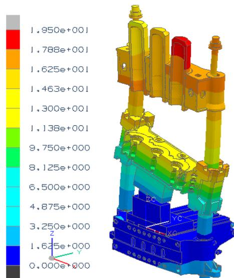
Figure 4. Frame displacement in the longitudinal direction
