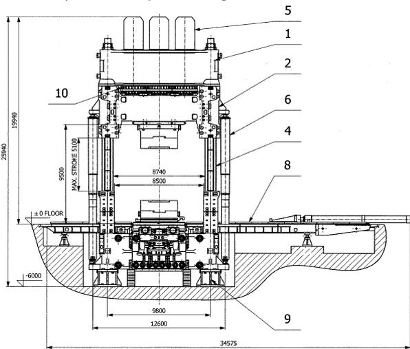
Figure 5. Design of the CKV 120/140 (SUNAN) press with the basic dimensions indicated (as viewed from the manipulator side)
