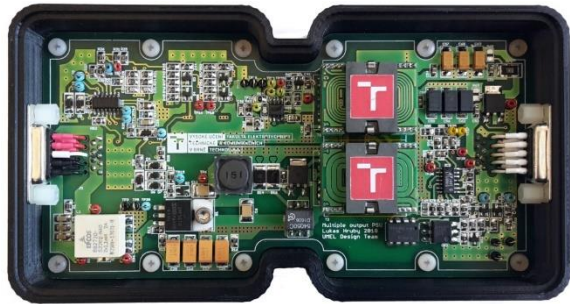
Figure 8: Power supply unit
