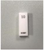
Fig. 3. 10mm ceramic gauge block
