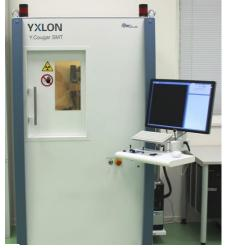
Fig. 2. X-ray, CT control system - Y. Cougar SMT
