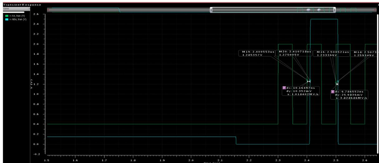
**Figure 46.** Delay of the address bit D0 for a capacitive load of 20pF and for a clock frequency of 10 MHz.
