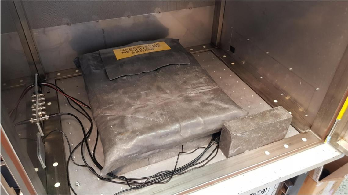
**Figure 81.** Complete shielding used during the measurements of XRF and gamma photons.
