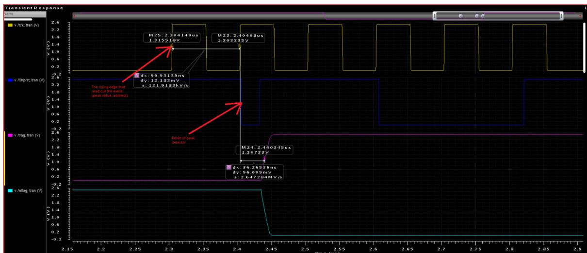
**Figure 66.** Simulation of the flag delay after clock edge to lower. Provided by Wenbin Hou – BNL.
