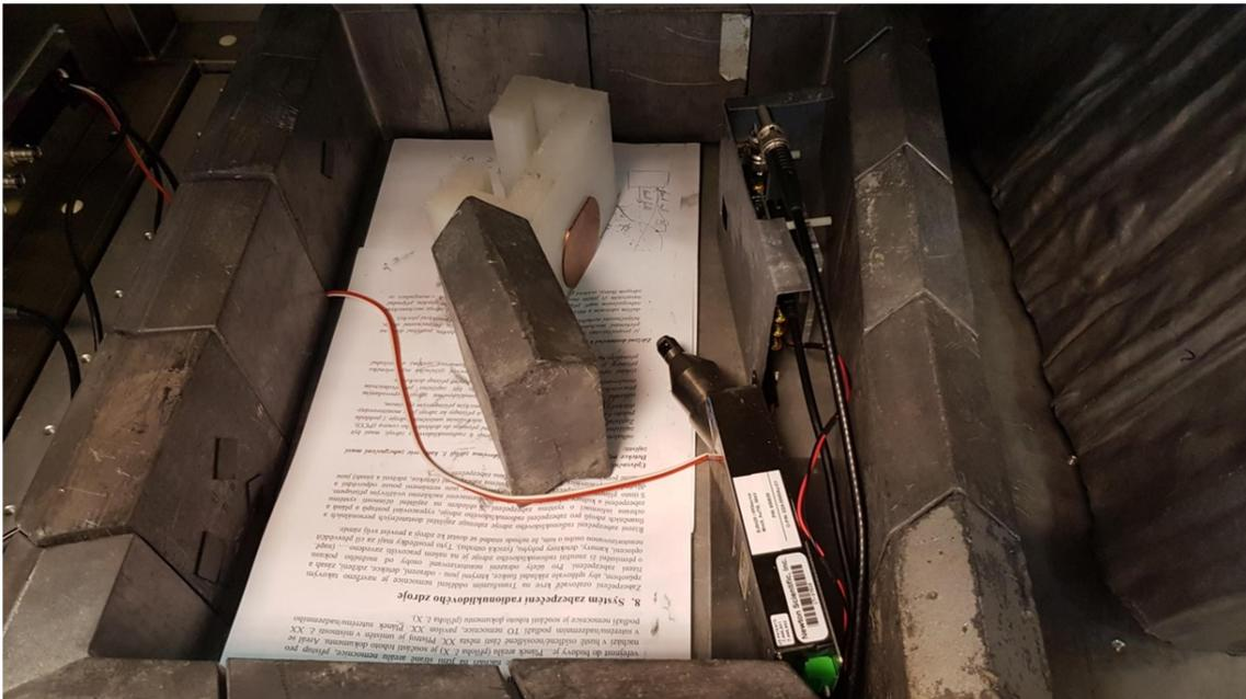
**Figure 80.** Setup used in the measuring of XRF. A mini X-ray tube (AmpTek) was utilized to obtain XRF below 30 keV.
