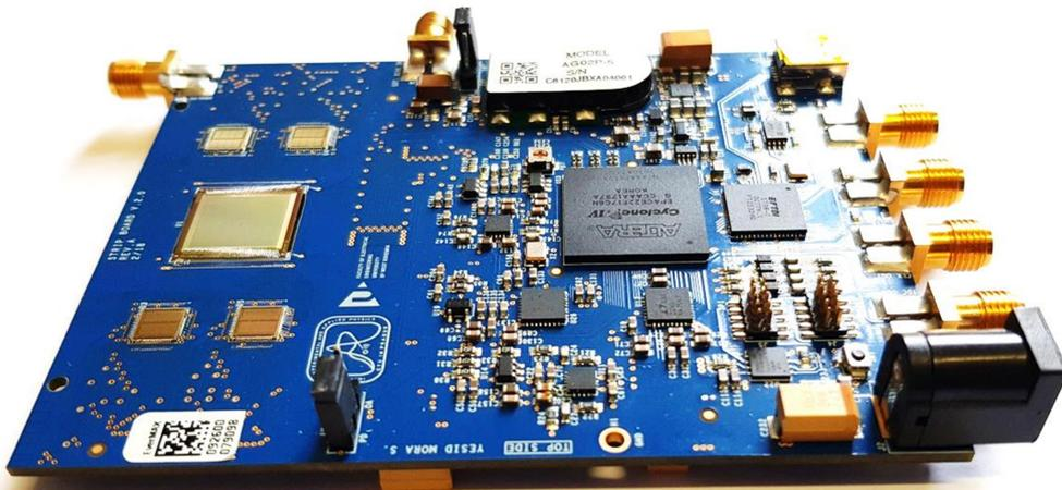
**Figure 58.** Second hardware version. It contains all the components in a single PCB.
