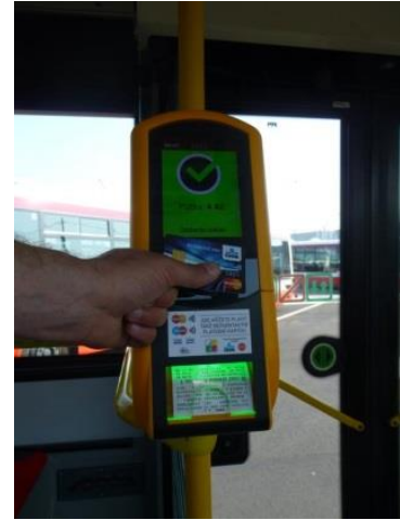
Figure 1: Ticket terminal accepting bank cards [21]
