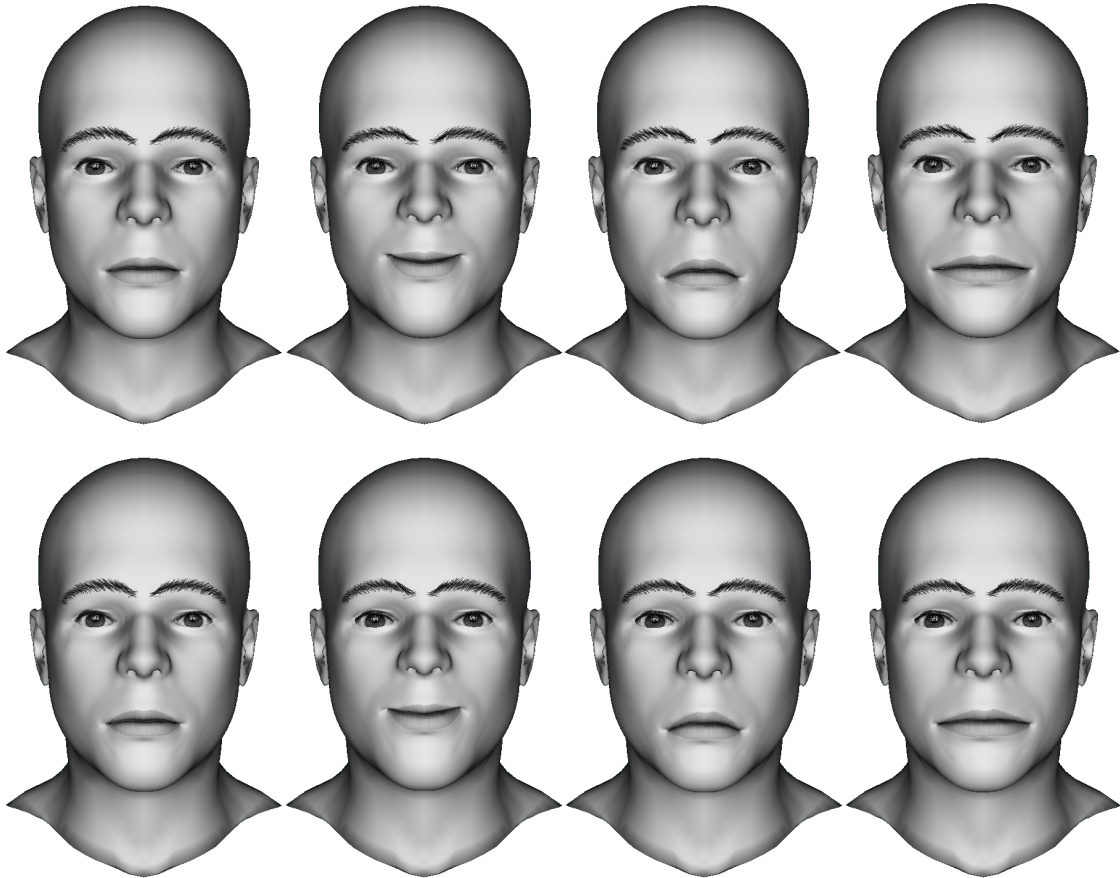
Figure 9.9: Head model deformation using feature points. Models created using manually inserted (top row) and automatically detected points (bottom row). Face expression (from left to right): original model, happy face, sad face, wide mouth.
