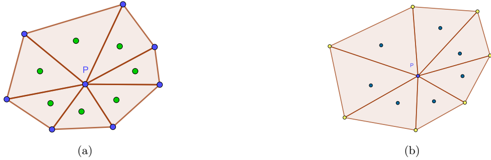
Figure 10.3: a) Point cloud P_i (blue points) as triangulation with green centroids of triangles; b) Points P_i of cloud (blue points) are used as centroids of “virtual” triangles. The yellow points are just for illustration of one possible “virtual” triangulation of the neighborhood.
