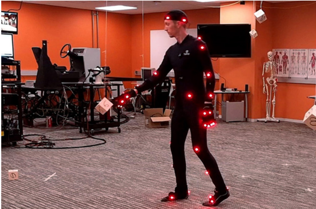
Figure 2.1: Modern active marker-based system, PhaseSpace
