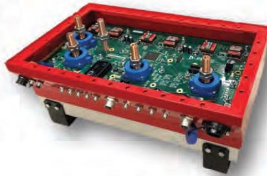
Figure 9. Control board with 3-phase inverter
