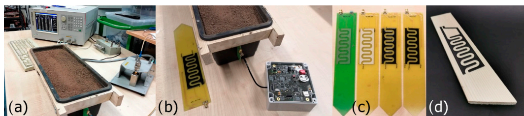
Figure 3. All soil moisture sensors were calibrated using both the (a) Agilent 4287A RF LCR Meter and (b) the developed Internet of Things (IoT) electronic measuring unit. (c) Image of Cu and printed soil moisture sensors, from left: Cu, AGS, CMD, CSP. (d) Wood plank-based sensor CMD/plank.
