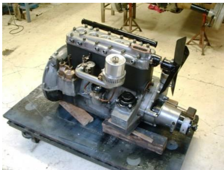
Obr. 7: Motor Praga Alfa 1496ccm [13]
