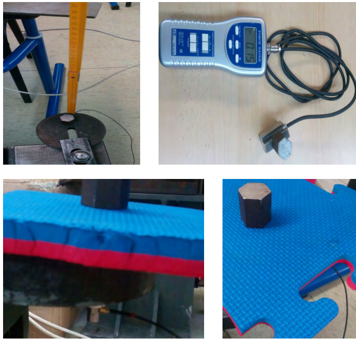
Figure 25. a, b, c, d – The height of the fall of the object is 35 cm, the mass of the object is 0.15 kg (150 g). Total workplace with added oscilloscope
