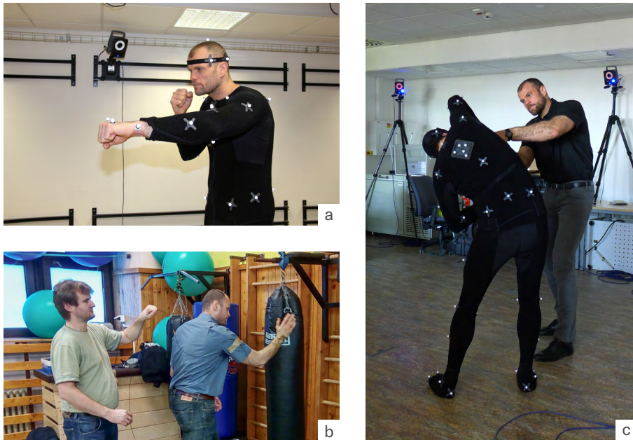
Figure 17. a, b – connecting the sensor with a cable or kinematics markers can limit the athlete's movement during the measurement), c – in another measurement design, the measuring sensors also limit who performs the test on the measured athlete).
