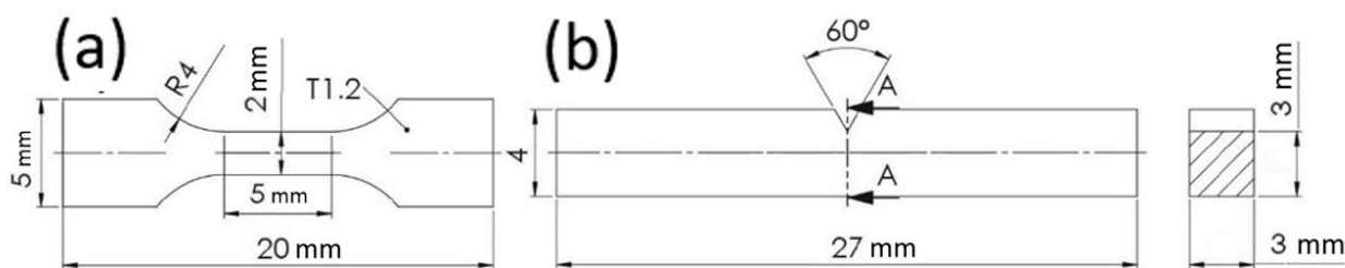
Figure 1. Samples for mechanical testing, (a) tensile test, (b) Charpy impact test.
