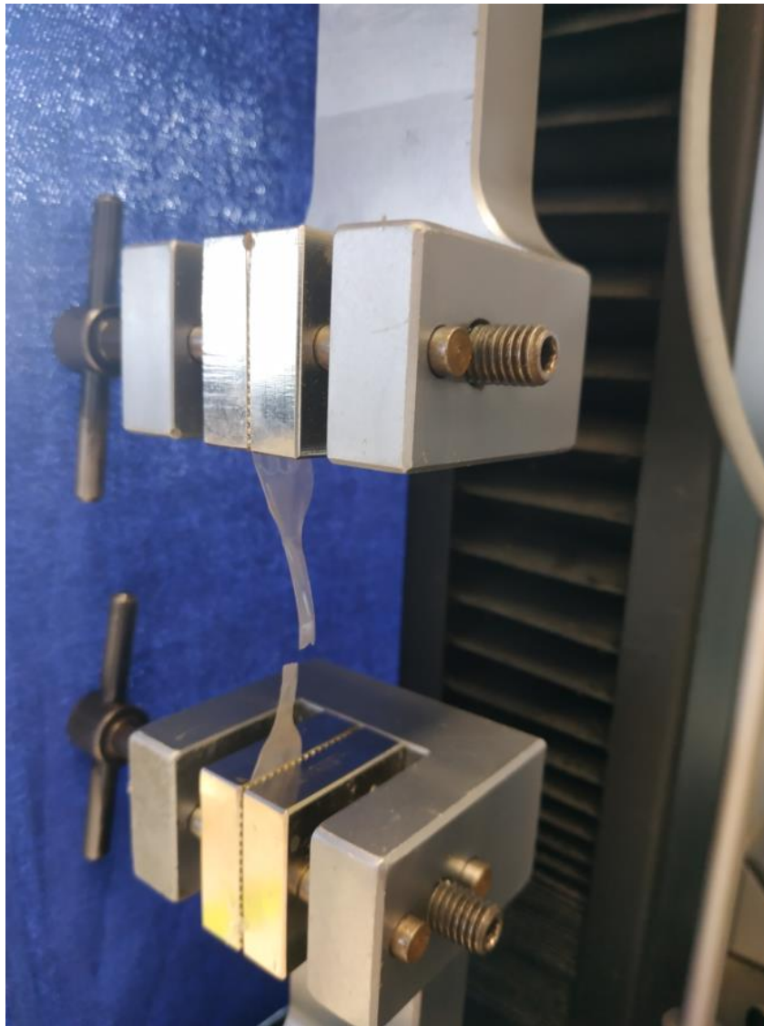
Picture 6.7 Mechanical test of PEN foil
