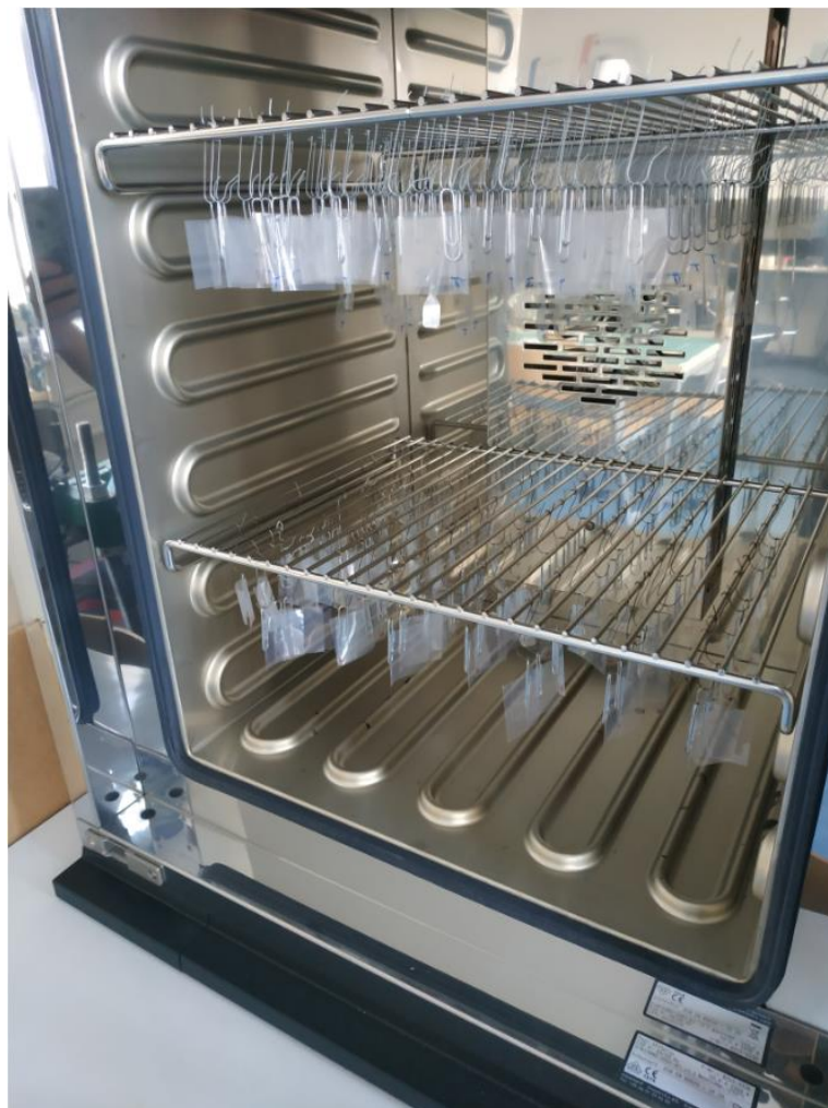
Picture 6.3 Thermal conditioning of PET and PEN films in an oven
