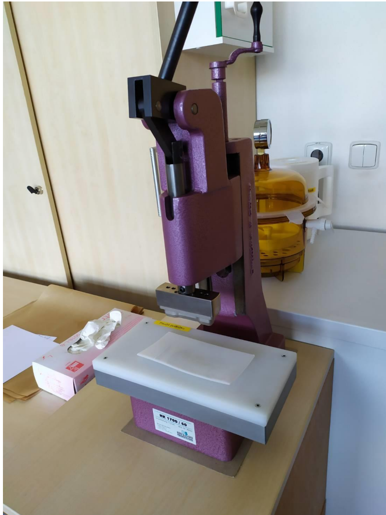
Picture 6.6 Press used in fabrication of test samples
