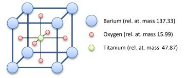
Fig. 1. Unite cell structure of barium titanate
