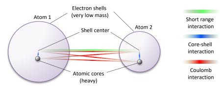
Fig. 2. Schematic representation of the core-shell model
