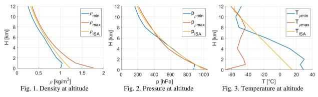
In used calculation model, the changing parameter of atmosphere is air density. Therefore, the extremes of density is used from handbook. Fig. 1 contains extremes of density at altitudes while Fig. 2 and Fig. 3 shows pressures and temperatures that occurs at this densities.
