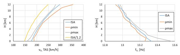
Fig. 7. ID3-DLM, flutter velocity at altitude
