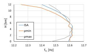
Fig. 6. ID3-2D, flutter frequency at altitude
