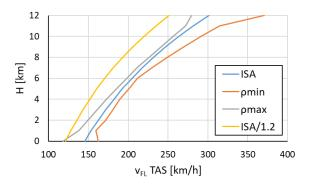
Fig. 5. ID3-2D, flutter velocity at altitude
