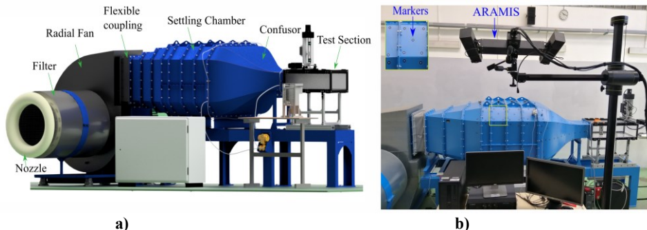
Fig. 1. Construction of the wind tunnel and optical measuring system ARAMIS. a) General view of the wind tunnel. b) Analysis of structural deformation of the wind tunnel.
