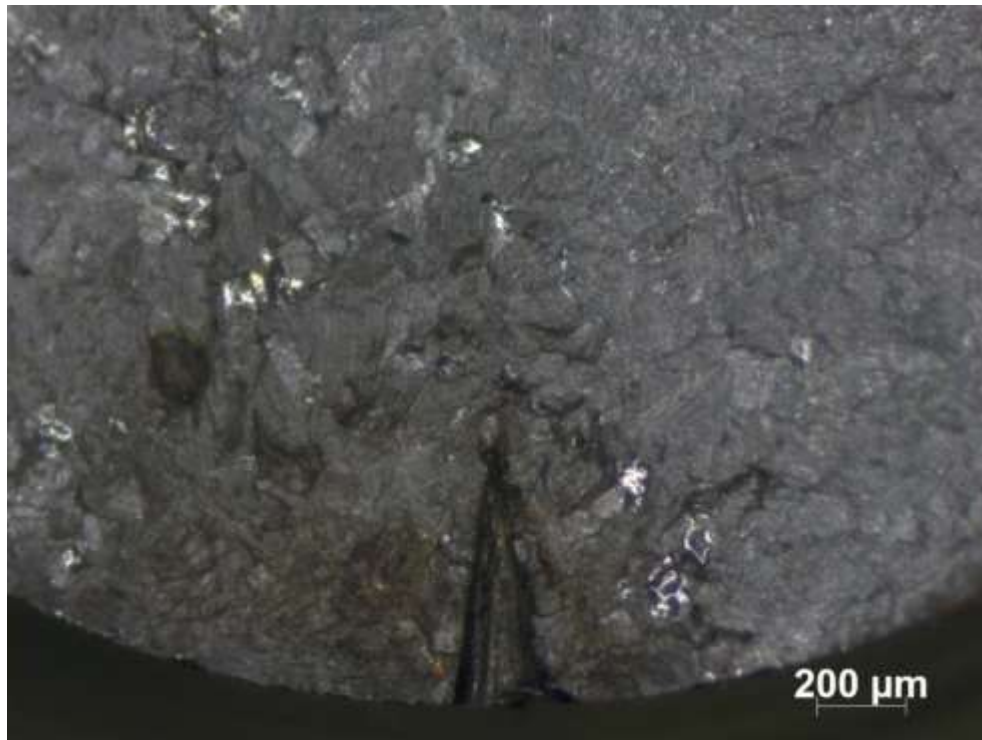
Obr. 12.11-3 Lomová plocha s vrubem
