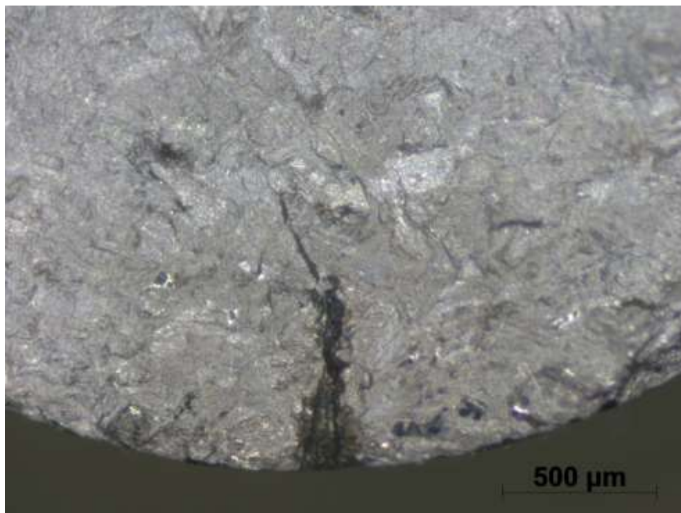
Obr. 12.8-3 Lomová plocha s vrubem
