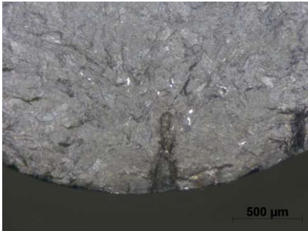
Obr. 12.7-3 Lomová plocha s vrubem
