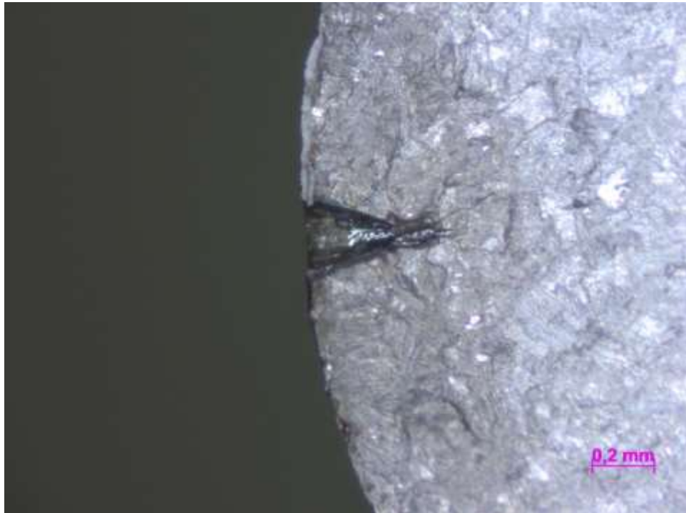
Obr. 12.5-3 Lomová plocha s vrubem
