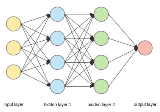
Figure 4.3: Example of standard neural network. The network has one input layer, two hidden layers, and one output layer. [16]
