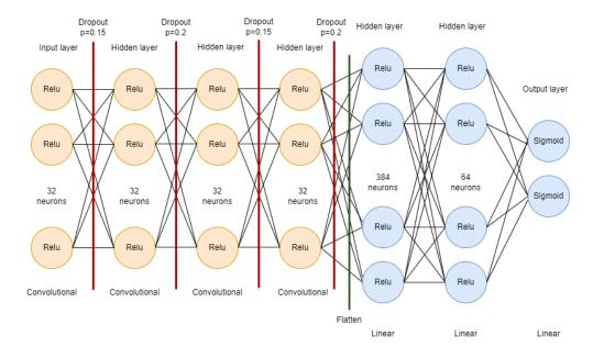
Figure 9.1: The CNN neural network net. Dropout layer prevents stuck in the local minimum; Flatten is the link between CNN and Linear layer.
