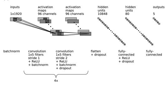
Figure 3.1: Network architecture. The feature extractor consists of eight convolutional layers, and the output of the last convolutional layer is flattened (Flatten). EEG time series data is batch normalized (Batchnorm) before the first convolutional layer is applied. The classifier consists of two fully connected layers. A softmax layer translates the activations of the previous layer into class probabilities. [7]
