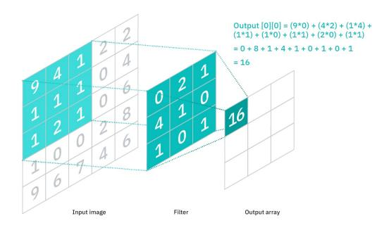
Figure 4.5: Application of filter on an image inside a CNN network. [5]
