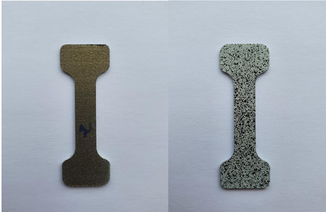
Fig. 36 Tensile specimen; left: as manufactured, right: prepared for DIC
