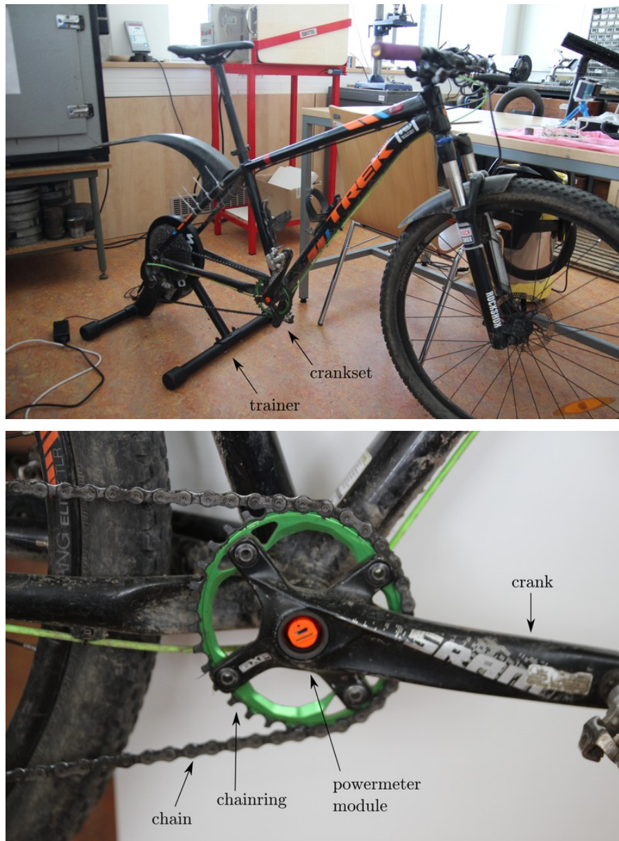
Fig. 6: The bicycle and indoor trainer as used for validation (top). Close-up on the installed powermeter with the watertight end cap removed (bottom).
