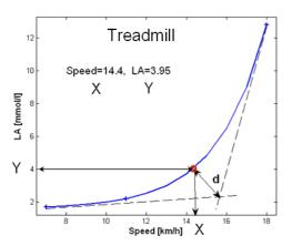
Fig. 4. Example of lactate curve and AnT (14.6 km/h) found after examination on treadmill ergometer. The curve is determined by 3 measured values of speed and lactate
