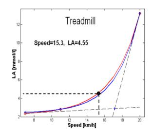
Fig. 8. Approximation from 2 LA measurements and 1 estimation value (red points, red curve). Approximation from 3 LA measurements (blue points, blue curve). See Tab. 1 for values
