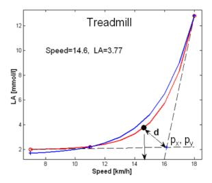
Fig. 6. Example of lactate curves for different initial values on treadmill ergometer. The correct AnT values are [Load = 14.6 km/h, LA= 3.77 mmol/l]. Measured - blue curve, Approximation from 3 lactate measurements - Red curve
