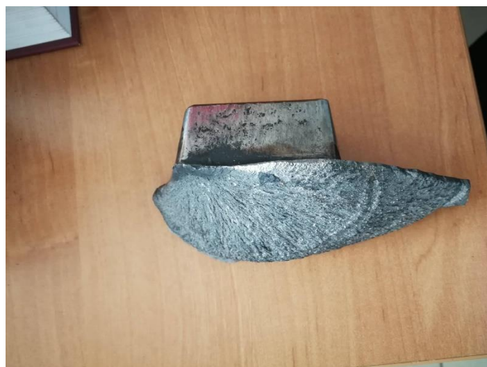
Fig. 1. Broken part of forging die
