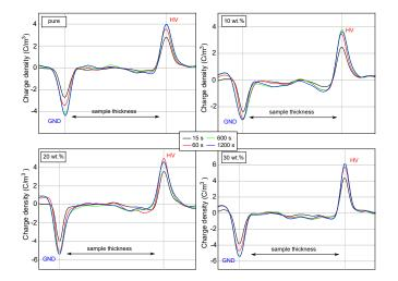
Fig. 4. Space charge distribution for different wt.% of EP/MgO composites in comparison with pure EP.
