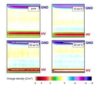
Fig. 3. PEA space charge patterns for different wt.% of EP/MgO composites in comparison with pure EP.
