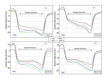
Fig. 5. Electric field distribution for different wt.% of EP/MgO composites in comparison with pure EP.
