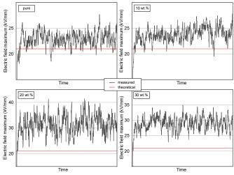
Fig. 6. Maximum electric field in time for different wt.% of EP/MgO composites in comparison with pure EP and with theoretical electric field.
