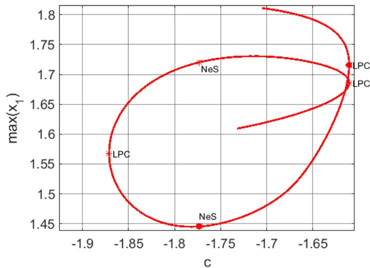
Fig. 5. Bifurcation diagram of the periodic orbit of system (26) as a function of the parameter  $c$  plotted against the  $\max(x_1)$
