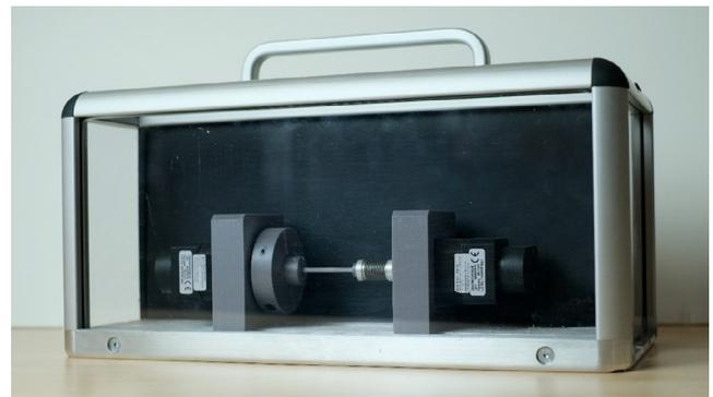
Fig. 1. Motion setup: mechanically coupled 2DoF system
