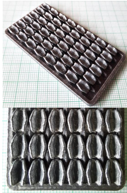
Figure 5 Printed prototype, made of aluminum, 1mm pattern underlay
