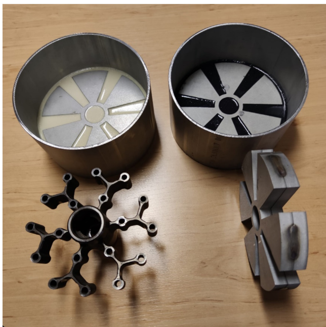
Fig. 17. Chemical junction – potting inside the plug and absorbers holder.
