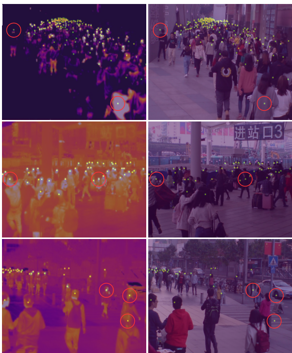
Figure 5: Illustration of the annotations (yellow squares) of the RGBT-CC [Liu21] dataset for both modalities. It can be seen that the annotations were created based on the thermal images. For better understanding, examples of inaccuracies in the annotation of the optical images have been encircled. The thermal images are also encircled in the corresponding places, but the annotations are correct there.
