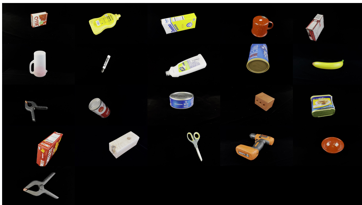
Figure 1: A qualitative sample of all 21 YCB-V objects, that were recorded with a handheld smartphone and our proposed black background. It can be seen that the objects are well silhouetted against the background and can therefore be segmented in an easy way and many typical chroma key-associated problems are circumvented.
