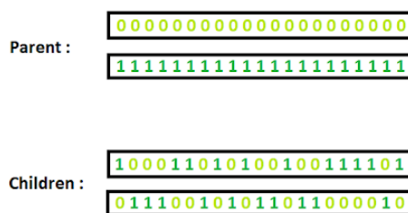
Figure 3: Graph of the uniform crossover with two parents and two offsprings
