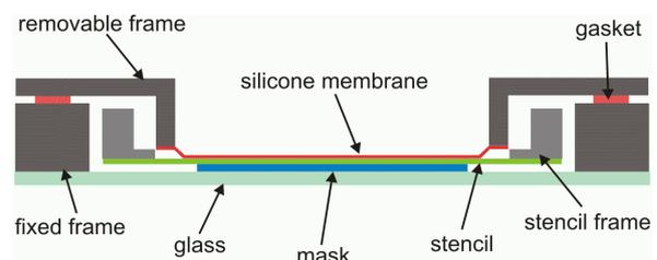
Fig. 2. Vacuum fixation system of exposure equipment.
