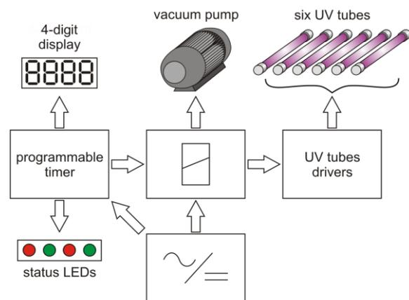
Fig. 1. Exposure equipment block scheme.
