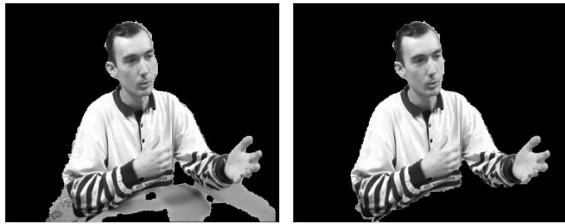
YUV foreground/background segmentation without (left) and with (right) shadow detection Figure 6:
