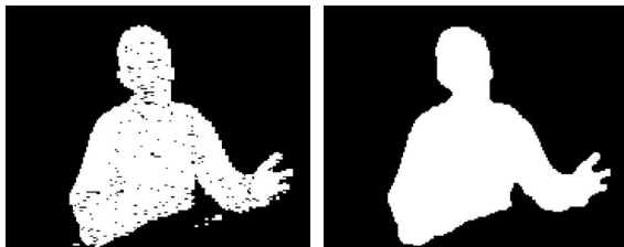
YUV segmentation mask without (left) and with (right) morphological Figure 7
