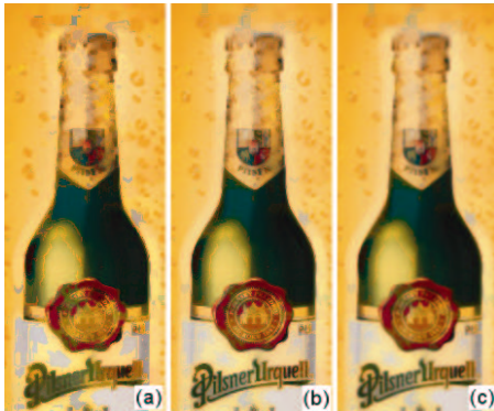
Morphological median – frame of the morphing sequence (a); after temporal linear filtering (b); and after spatial and temporal filtering (c).
