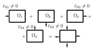
Fig. 2. Schematic procedure of computing rectangular cavities with non-zero boundary conditions on all sides
