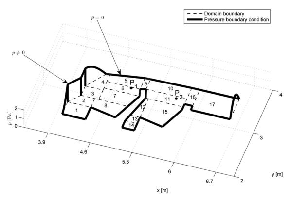
Fig. 4. Course of acoustic pressure boundary conditions. Points  $P_1$  and  $P_2$  are depicted as well as the interior boundaries of individual domains
