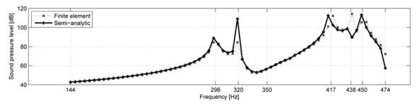
Fig. 10. Transfer functions of the acoustic pressure in the point  $P_2$
