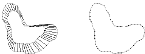
Figure 2: Matching between objects Foot1 and Foot2 using the local matching solution and applying the estimated rigid transformation without and with the scale factor, respectively.
